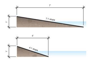
Beach slope is a critical component of a successful restoration project. A well-designed slope provides resistance to erosion, reducing the need for maintenance. Slopes of 7:1 or flatter are ideal (seven horizontal feet for each vertical foot), but slopes up to 4:1 can be stable in some circumstances.
